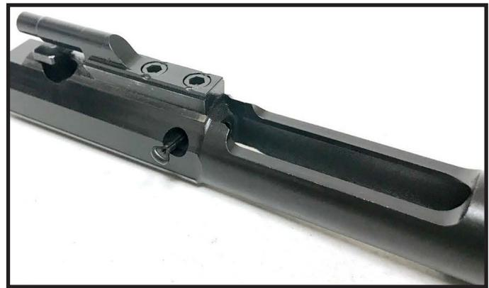
8. Tilt the bolt face up and remove the firing pin.
