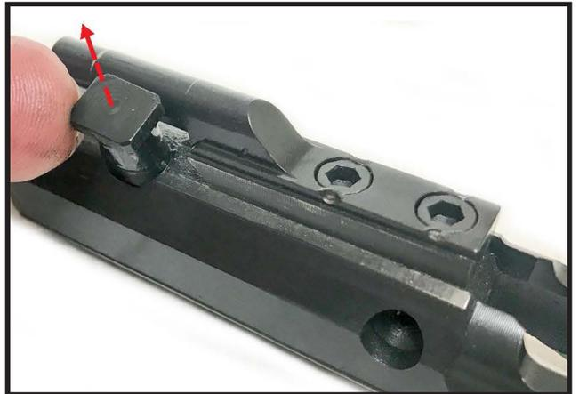
11. Pull the bolt forward and remove it from the bolt carrier.
