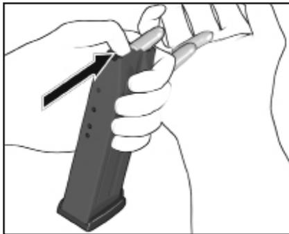
Figure 26 — Unloading magazine
