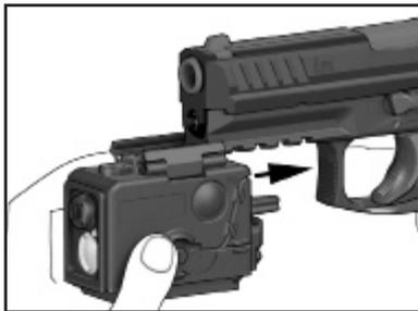
Figure 53 — Installing accessory onto the rails
