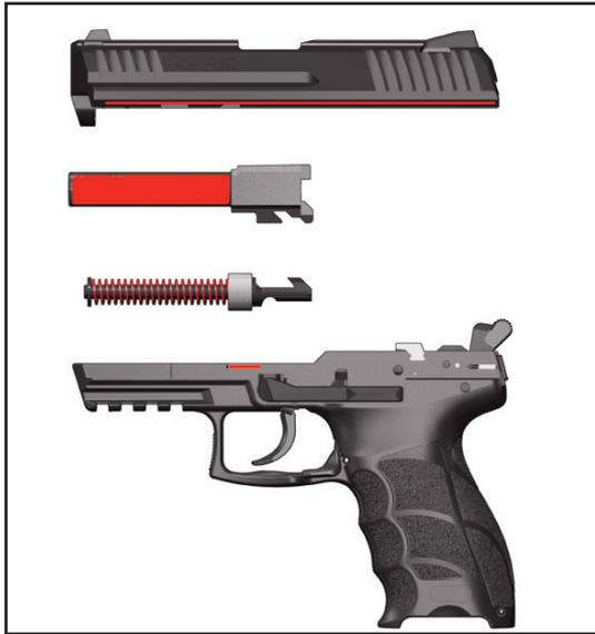
Figure 47 — Lubrications Points (in red)
