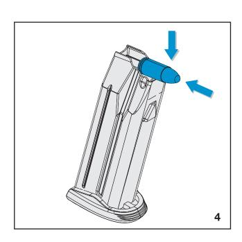
Hold the magazine in one hand. With the other hand, place a cartridge on the magazine follower in front of the feed lips at the top of the magazine. Press the cartridge down onto the follower and slide the cartridge under the feed lips until it is seated fully inside the magazine body.
